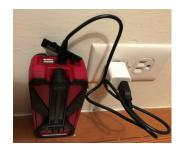
If the battery is flat, insert the adapter into the receptacle at the end of the radio and then plug the other end into a USB outlet in a plug. See the photo. The adapters for the radios given out before mid 2017 plug directly into a wall outlet and take several hours to recharge. (I left mine overnight.) The newer radios can also be recharged by plugging them into the USB port of any device with a charged battery, such as a computer, laptop or USB car lighter adapter.
